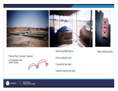
And basically what they do is they actually prepare the mixture of this, mixing with the cement 5% to 7% of the cement and to stabilize it and then they actually this is a mould process. So, they keep that and then they press it and then these moulds will come out of it and this is where the interlocking bricks because these are very helpful for having a vertical reinforcement at the corners or the junctions.
